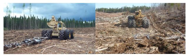
Figure 5-7: Site preparation of a cutover using shark-fin barrels and anchor chains.
